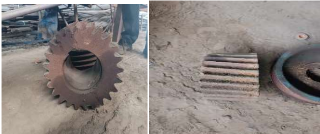
HELICAL PINION GEAR OD - 264mm ID - 120mm KEY WAY- 30x12mm NO OF TEETH- 24 Nos FACE WIDTH - 155mm TOTAL WEIGHT - 10 Kgs
