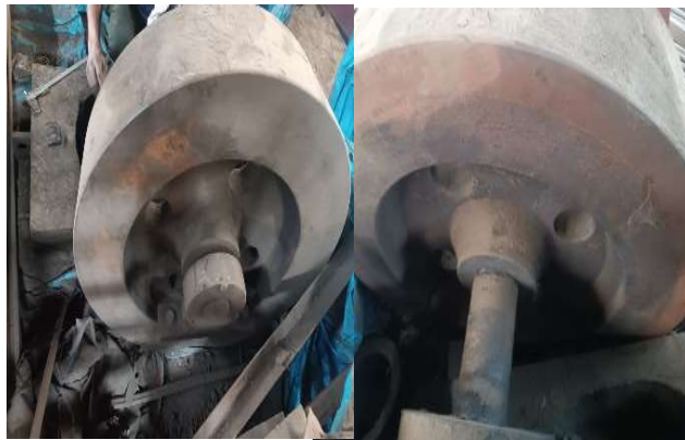
FLYWHEEL OD - 1050mm ID - 120mm FACE WIDTH - 255mm TOTAL WEIGHT - 2500 Kgs
