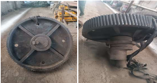
HELICAL GEAR OD - 1090mm ID - 216mm KEY WAY- 50x20mm NO OF TEETH- 106 Nos FACE WIDTH - 150mm TOTAL WEIGHT - 1000 Kgs
