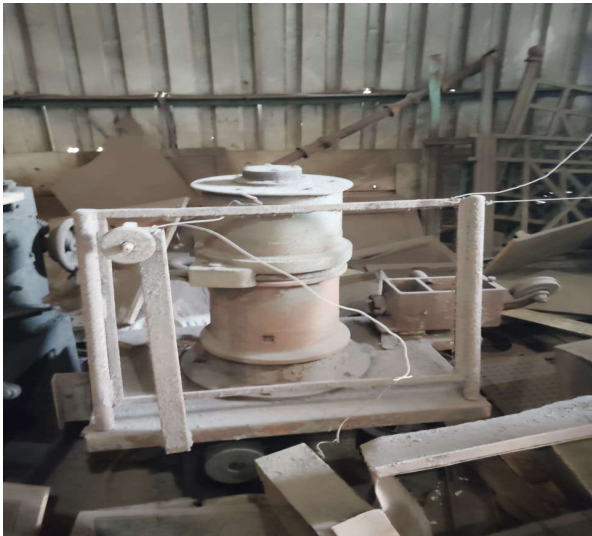
Co2 WIRE DRAWING DRUM ASEMBLY WITH GEAR BODY DRUM SIZE-600mm MACHINE DIMENTION- 1400mmX1200mm TOTAL WEIGHT -250 Kgs
